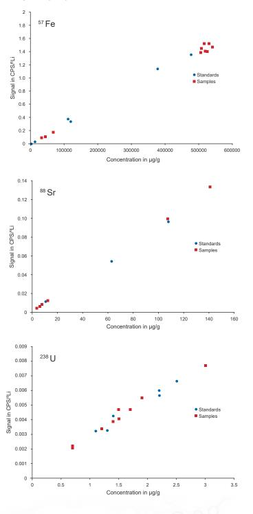
Figure 2. Shows the linear calibrations that can be achieved using the LA-ICPMS technique. The blue markers represent the calibration standards, while the red markers are unknown samples where the determined concentration has been plotted against the predetermined value from solution ICPMS. Where a predetermined value was not provided the data has not been plotted. The majority of calibration plots have coefficients of correlation >0.95.
