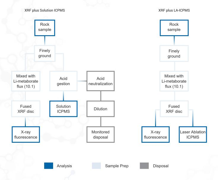
Figure 1. Compares the work flows for the solution-digestion method and the new LA-ICPMS method. The method completely removes an entire sample preparation stream, thereby saving consumables, reducing man hours per sample and improving environmental credentials for the analysis.
